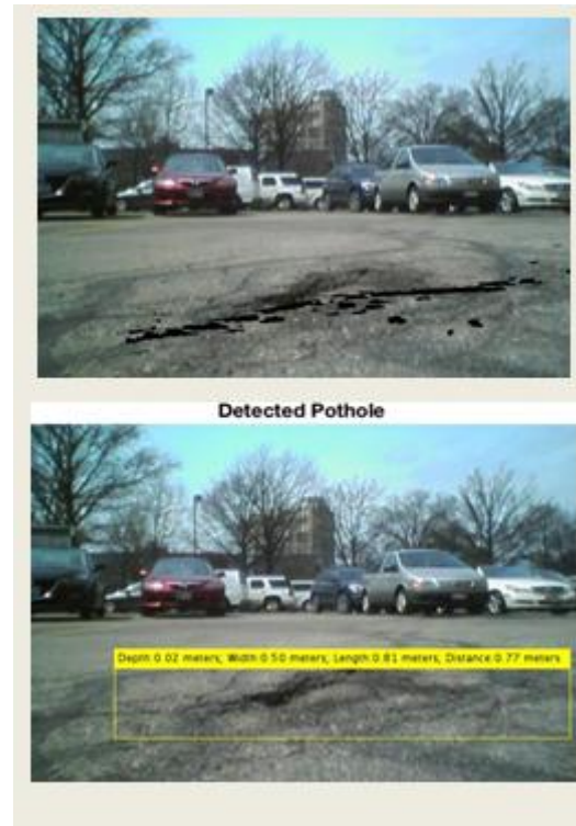
Fig. 11.The Experimental Setup for Pothole Detection.
