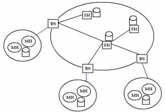
Large databases can run on servers that guarantee efficient processing and reliable storage of database. Fixed hosts perform the transaction and data management functions with the help of data base servers (DBS). Mobile units are the portable computers which can retain the network connections through the support of the Base Stations (BS).
