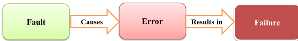
Fig - The path to failure
